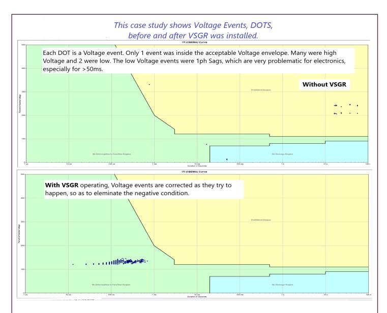
In a recent case study, we captured Voltage events before and after **VSGR** (Voltage Stabilizing Ground Reference) was installed.
